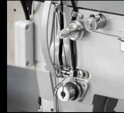
Upper thread tension monitoring Skipped stitches detection, thread breakage detection, dynamic upper thread tension monitoring.
