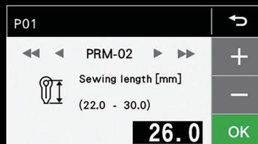
The maximum and minimum setting range of the sewing length is described, making it easy to change the setting.
