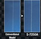
Short remaining thread, (3mm) doesn't require after-cutting process
