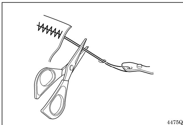
2. If the upper thread trailing length is 40 mm or more, or if the upper thread tension is weak and the upper thread does not form a good seam at the first stitch, the end of the thread that is being held by the thread nipper may become wound around the seam. Furthermore, if using thick thread that is #30 or higher or if the thread trailing length is too long, an error [E691] may occur. In any of these cases, use scissors to cut the thread without pulling it up too hard.
