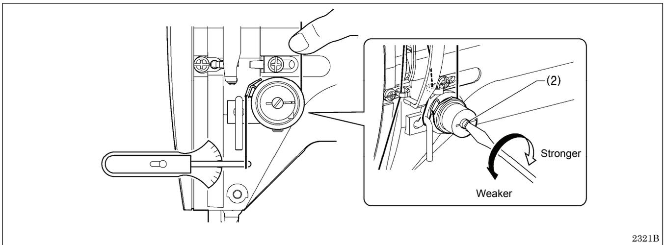
Adjust by turning the shaft (2) with a screwdriver.
