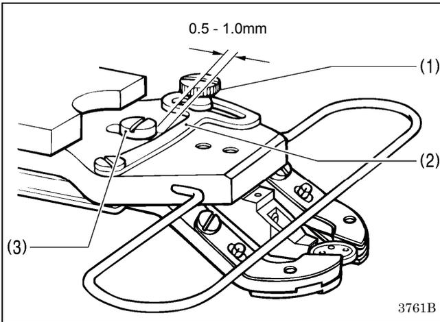
1. Insert the button in the button clamp, and then confirm that the button is securely held by the clamp and that the button can be turned by hand.
