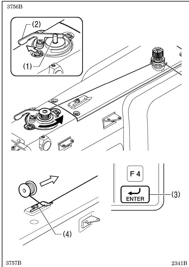
1. Place the bobbin onto the bobbin winder shaft (1).
