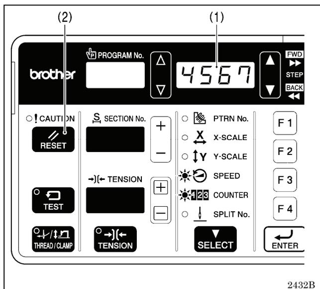
1. The counter is incremented by 1 each time one sewing operation is complete. If the production counter display is active, the number being displayed in the menu display (1) will be incremented by 1.
