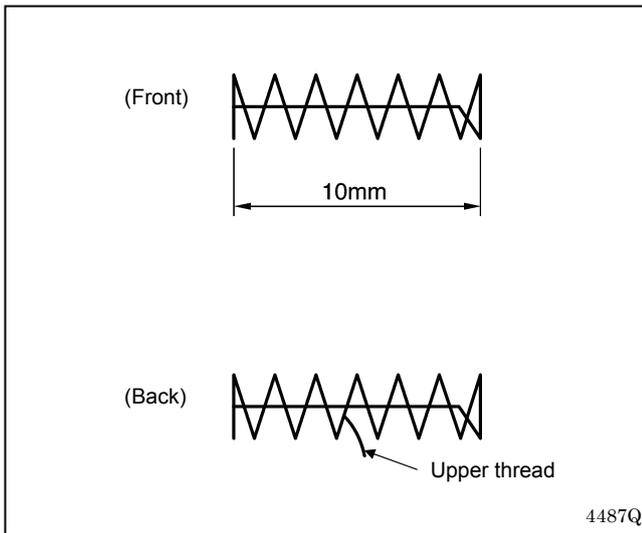
3. For sewing patterns with a short bar tack length (10 mm or less), the end of the thread that is being held by the thread nipper may poke out from the seam on the underside of the material. It is recommended that you change the thread nipper setting to "OFF" for patterns such as these.
