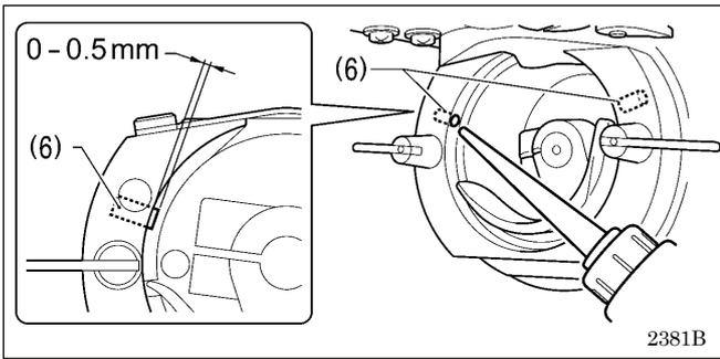
7. Pour oil in through the two holes of the shuttle race base assembly so that the felt (6) is lightly moistened.
