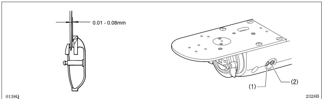
Turn the pulley to align the tip of the rotary hook with the needle center line. Then loosen the set screw (1) and turn the eccentric shaft (2) to adjust so that the clearance between the needle and the rotary hook is 0.01 - 0.08 mm.
