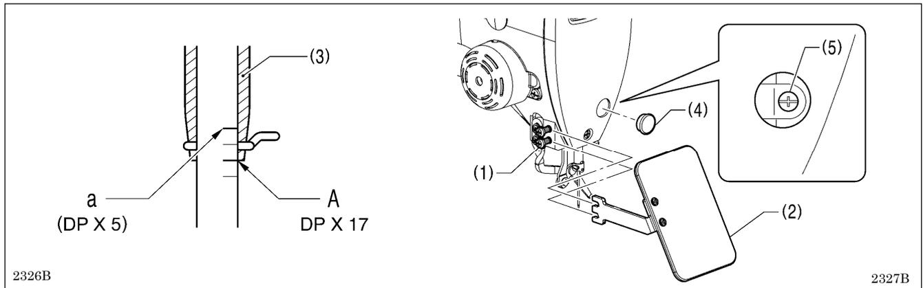
1. Loosen the two screws (1), and then remove the eye guard assembly (2).
