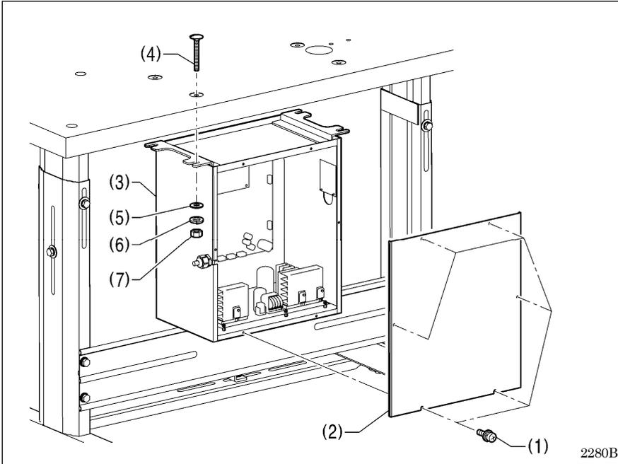
Remove the six screws (1), and then remove the control box cover (2).
