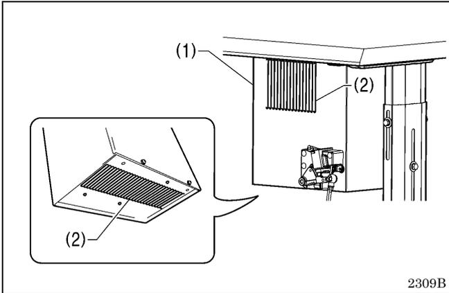
Use a vacuum cleaner to clean the filters in the air inlet ports (2) of the control box (1) at least once a month.
