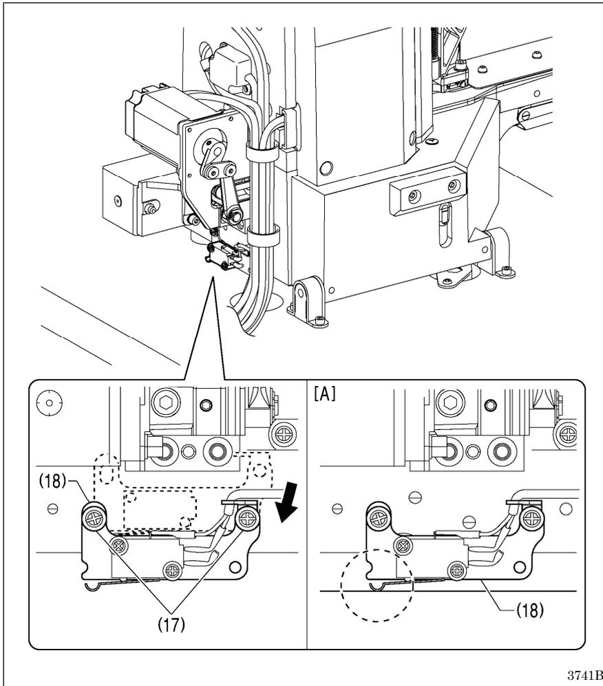
1. Remove the two screws (17), and then temporarily remove the machine head switch (18).
