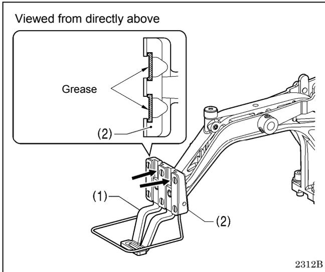
Periodically apply grease to the sliding parts of the work clamp (1) and the work clamp arm (2).
