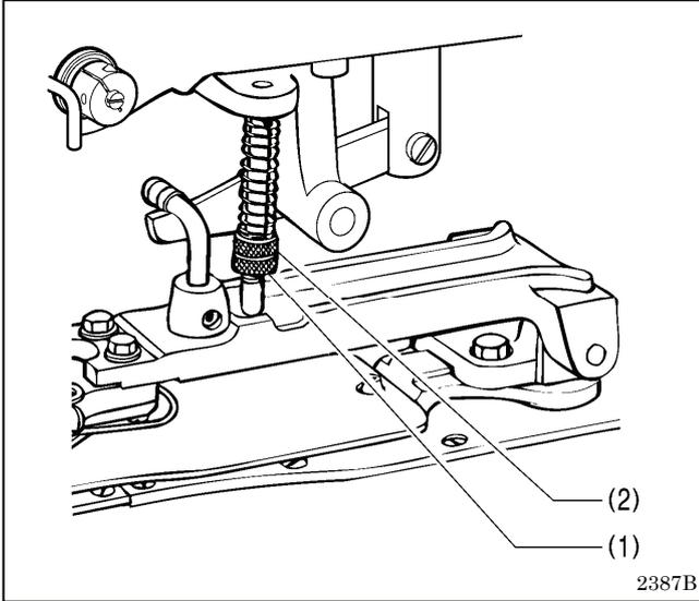
Loosen the nut (1) and turn the nut (2) to the point where it is just tight enough that the material will not slip out of place when it is slightly pulled (keep pressure as slight as possible).
