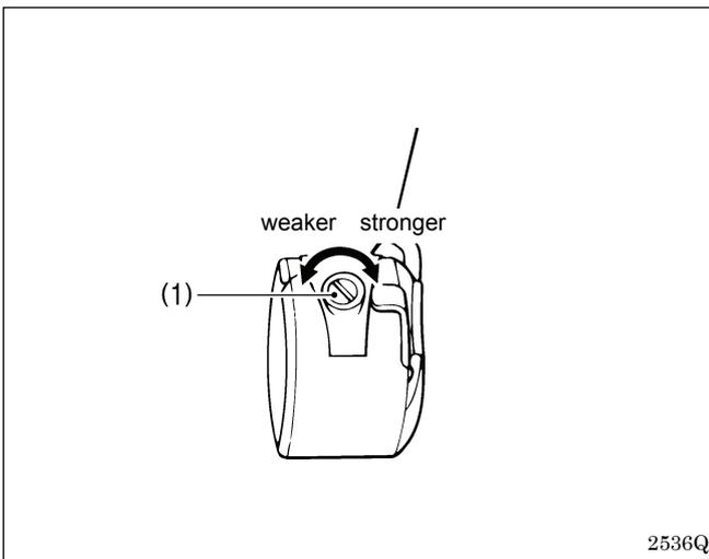
Adjust the thread tension to the weakest possible tension by turning the thread tension nut (1) until the bobbin case will not drop by its own weight while the thread end coming out of the bobbin case is held.
