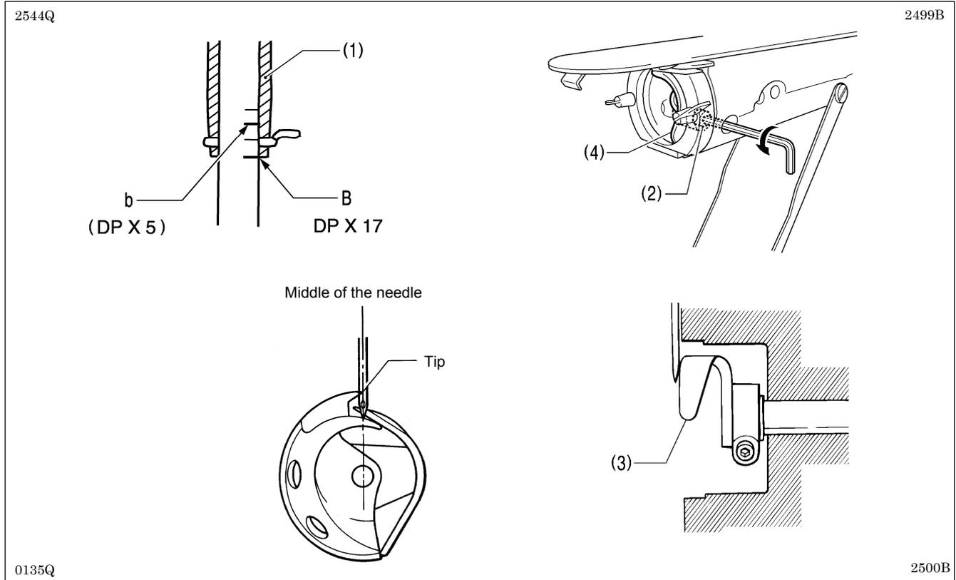
1. Turn the machine pulley to raise the needle bar from the lowest position until the lowest reference line on the needle bar (reference line B) is aligned with the lower edge of the needle bar bush (1).
