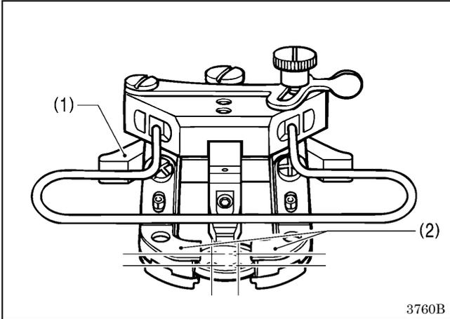
1. Press the button clamp plate cam (1) to open the button clamp (2).
