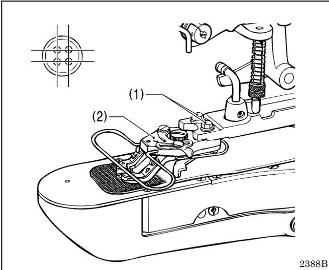
1. Loosen the two bolts (1) and adjust the button clamp base (2) by moving it.
