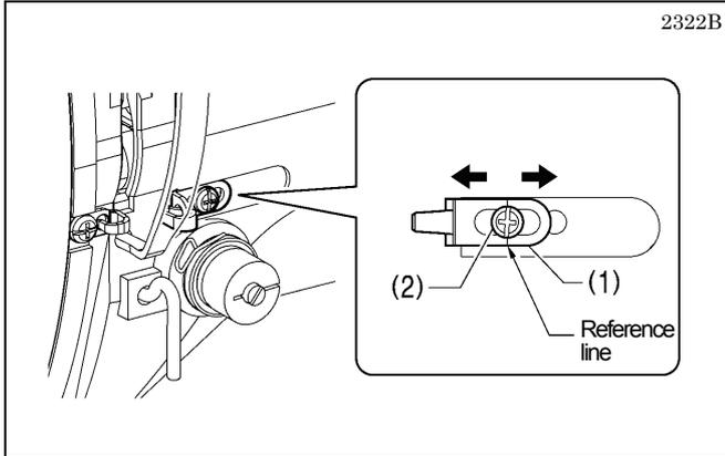
The standard position of arm thread guide C (1) is when the screw (2) is aligned with the position of the reference line. To adjust the position, loosen the screw (2) and then move arm thread guide C (1).
