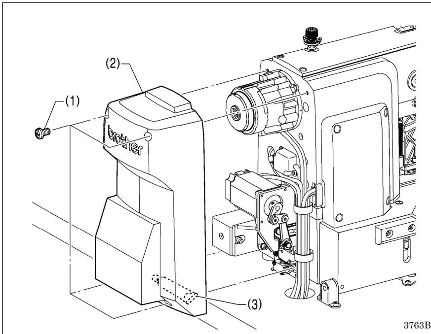
1. Remove the four screws (1), and then remove the rear cover (2).
