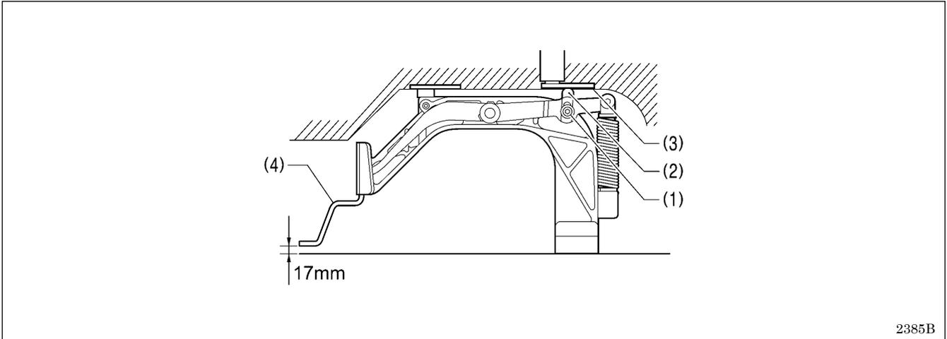
1. Loosen the bolt (1) and move the work clamp arm lever plate (2) up or down to adjust.
