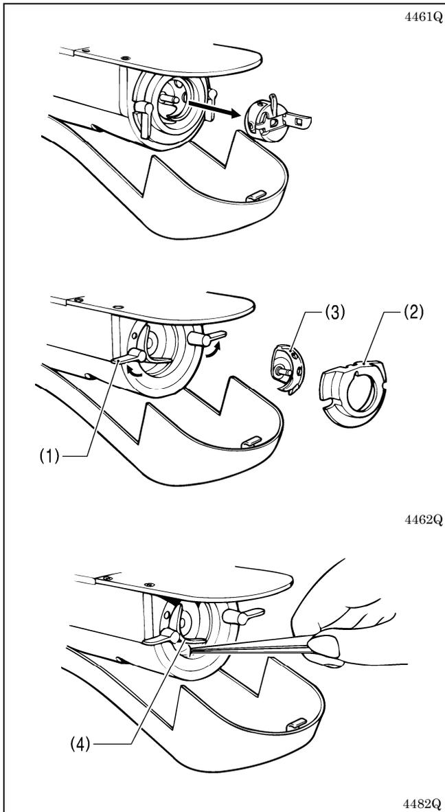
1. Pull the shuttle race cover downward to open it, and then remove the bobbin case.
