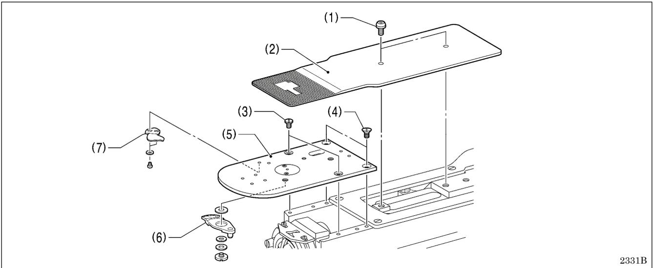
1. Open the shuttle race cover, remove the two screws (1), and then remove the feed plate (2).
