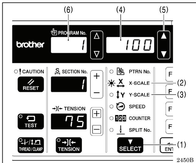
1. Press the SELECT key (1) so that the X-SCALE indicator (2) (for X-scale setting) or the Y-SCALE indicator (3) (for Y-scale setting) is illuminated.
