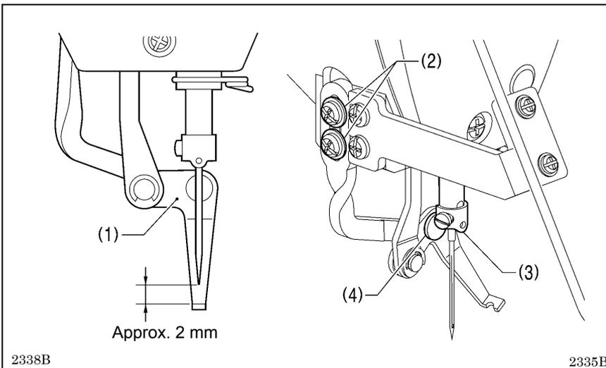
Loosen the two screws (2) and adjust the thread wiper (1) so that the clearance between the top of the thread wiper (1) and the needle point is approximately 2 mm when the thread wiper (1) is aligned with the center of the needle.
