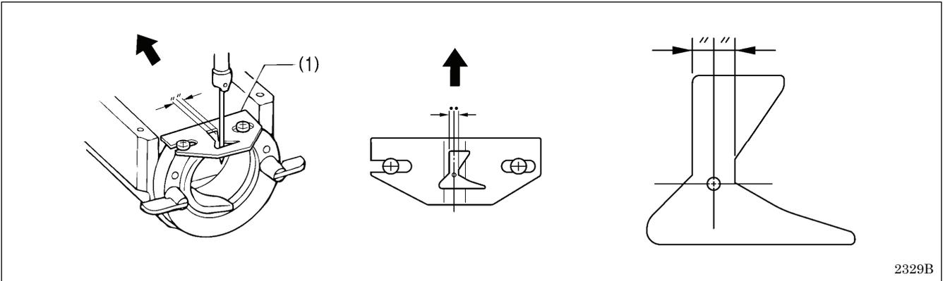
Install the shuttle race thread guide (1) by pushing it in the direction of the arrow so that the needle groove is aligned with the center of the needle plate hole.
