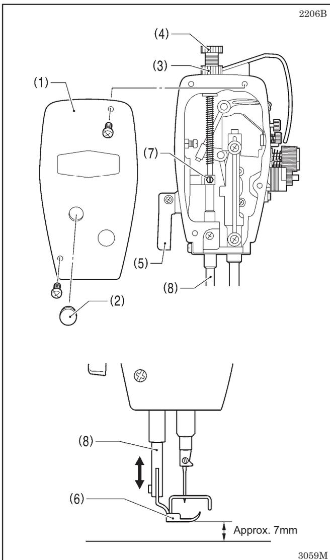
1. Remove the rear cover (1) and remove the rubber cap (2).
