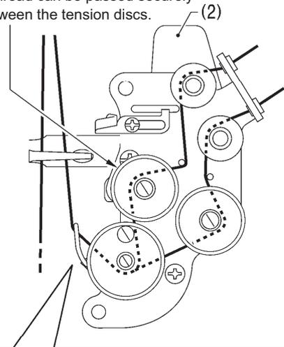
Pass the thread on the inside of the tab (3).
