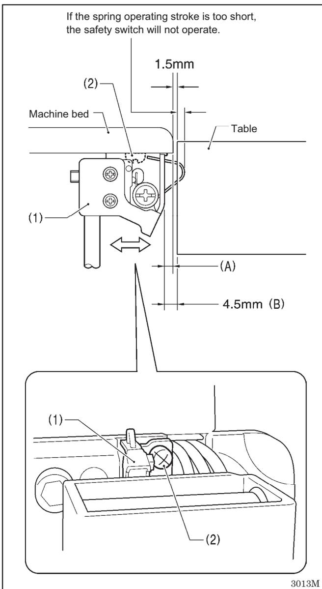
The standard installation position for the safety switch (1) is shown in the illustration at left.
