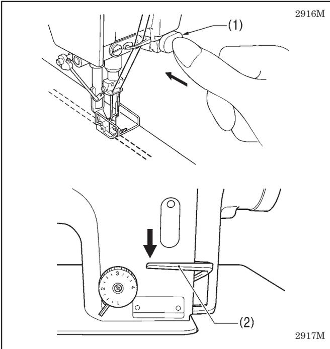
When the actuator switch (1) or the reverse lever (2) is pressed during sewing, the feed direction will be reversed. When it is released, the feed direction will return to normal.
