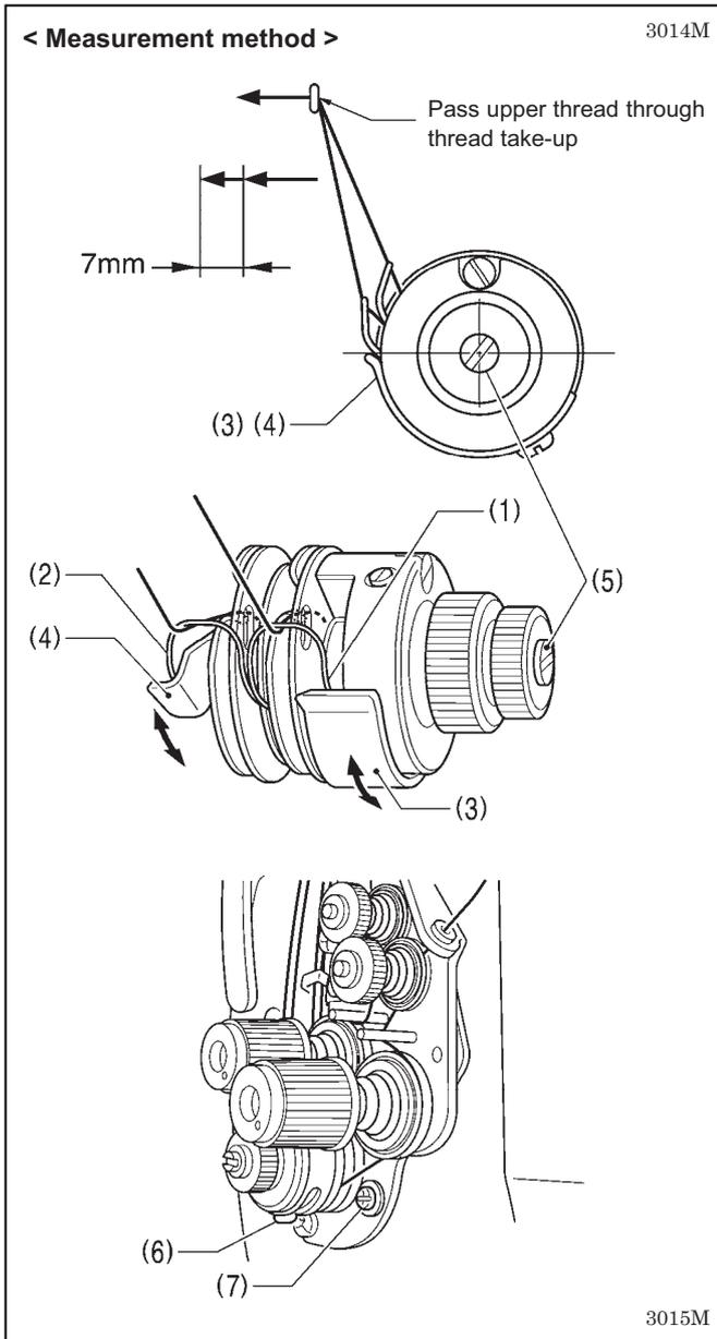
The standard thread take-up length for thread take-up springs R (1) and L (2) is 7 mm. You can adjust the thread take-up amounts by changing the heights of the stopper [right] (3) and the stopper [left] (4).
