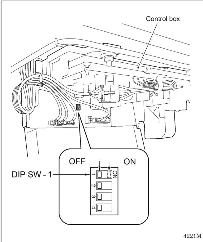
When the lock function is set to "ON", the key operations for making settings such as the following will be disabled in order to prevent these settings from being accidentally changed.
