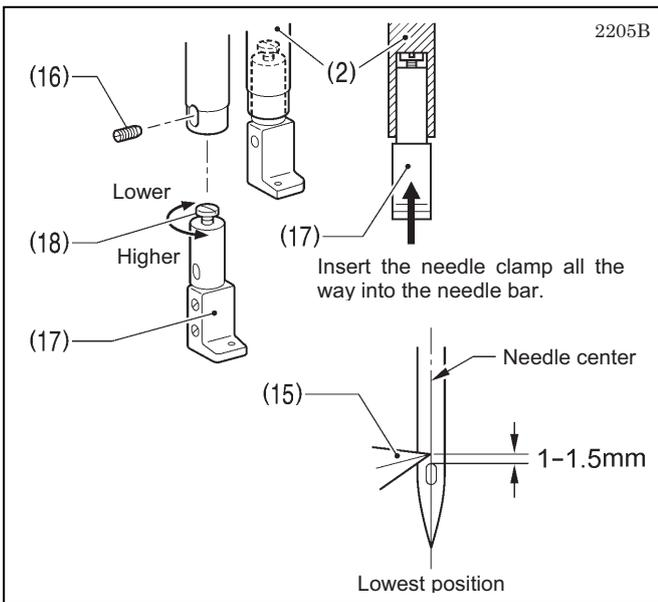
16. Loosen the set screw (16) and then pull the needle bar clamp (17) downward to remove it.
