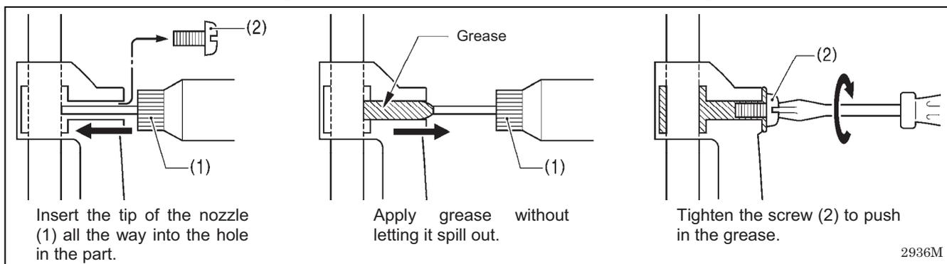
Insert the tip of the nozzle (1) all the way into the hole in the part.
