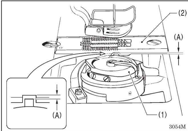
The clearance (A) between the rotary hook (1) and the needle plate (2) is adjusted as follows at the time of shipment from the factory.
