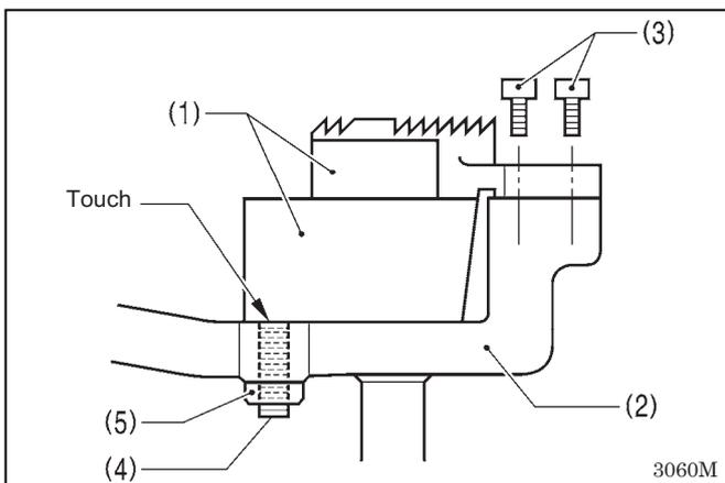
1. Install the feed dog (1) to the feed bar (2) with the two screws (3).
