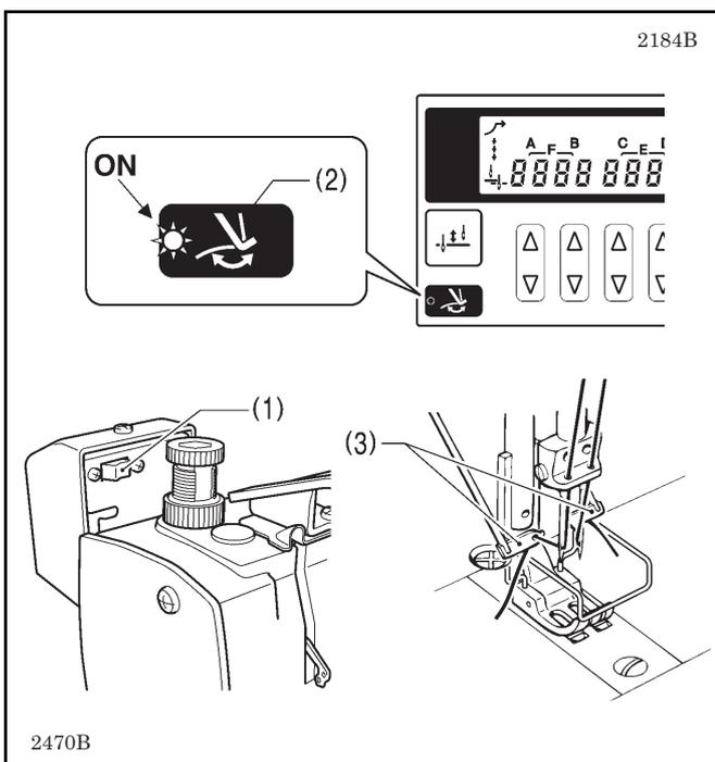
1. Press the thread wiper switch (1) to the  side.
