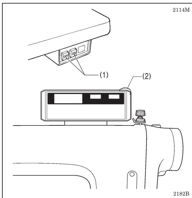
3. Press the ON power switch (1). The power indicator (2) will illuminate.
