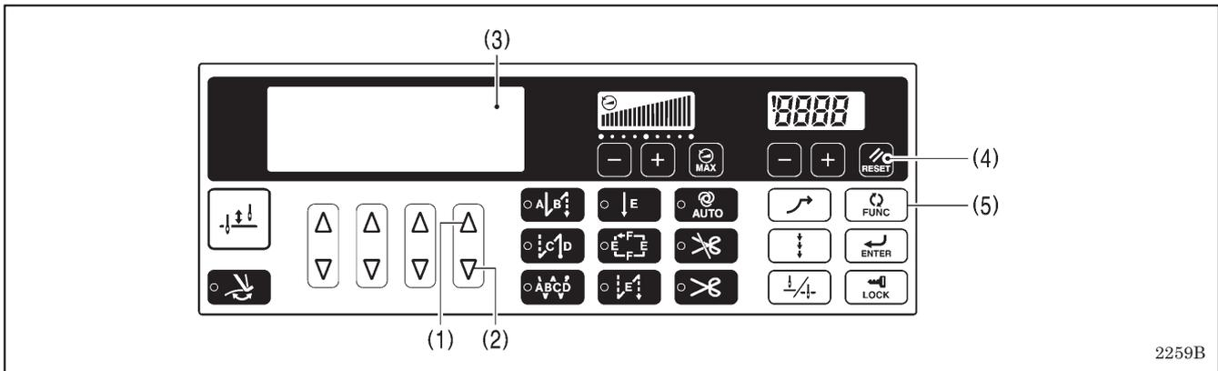
After the grease has been applied, carry out the following procedure to reset the grease consumption amount.
