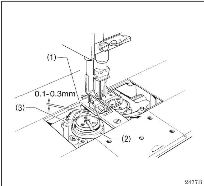
1. Loosen the set screw (3) and move the opener (1) to the left or right to adjust so that the clearance between the rotary hook (2) and the opener (1) is 0.1–0.3 mm when the opener (1) is pulled as far as it will go in the direction of the arrow.
