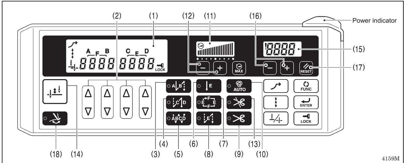
The power indicator illuminates when the power switch is turned on.
