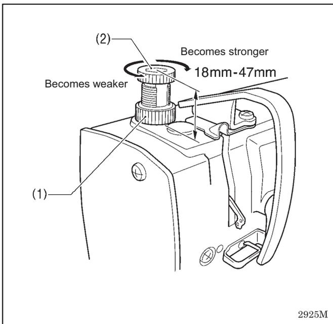
The presser foot pressure should be as weak as possible, but strong enough so that the material does not slip. (Refer to "Adjusting screw height" in the table below as a guide to adjustment.)
