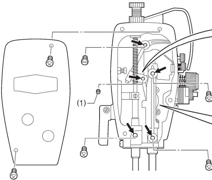
Turn the machine pulley until the screw (1) can be seen.
