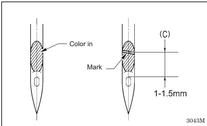
13. Use an oil-based marker pen to color in the hollow of the needle.
