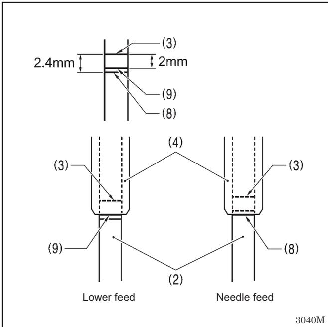
6. Turn the machine pulley forward to raise the needle bar (2) until the reference line ((8) or (9), depending on the feed condition) on the needle bar (2) is aligned with the bottom edge of the needle bar base (4).
