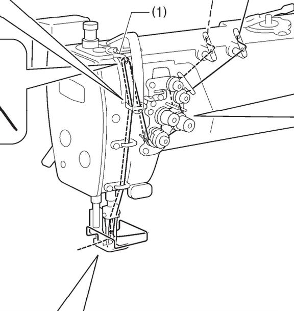
The thread can be passed securely in between the tension discs.
