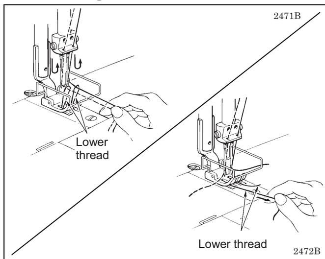
1. While holding the two upper threads with your fingers, turn the machine pulley by hand toward you until the lower threads come out onto the feed dog.
