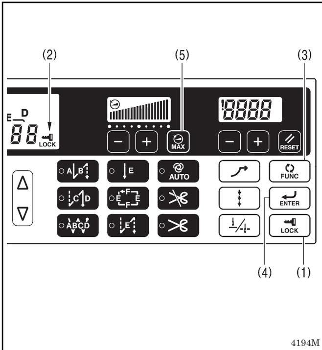
When the power switch is turned on, the LOCK key (1) turns ON. (The icon (2) is illuminated.) In this state, the following three key operations are disabled so that the setting values cannot be changed accidentally.
