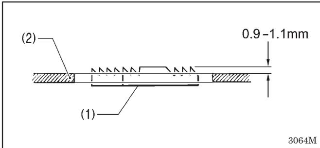
Turn the machine pulley forward until the feed dog (1) is at its highest position, and then adjust so that the feed dog (1) protrudes 0.9–1.1 mm from the top of the needle plate (2).
