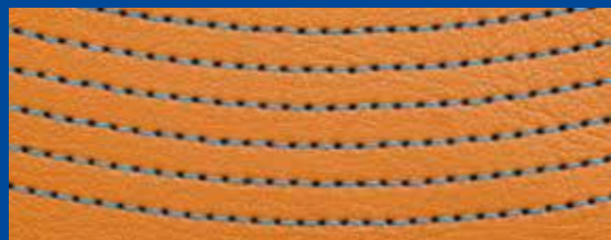
Sewing speed: 2,700stl/min stitch length: 3mm
